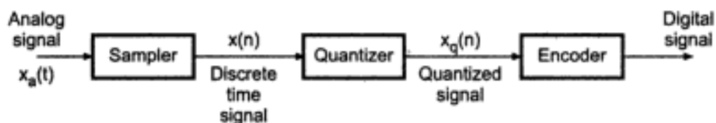
Fig. 2.10.1 Basic block diagram of A/D converter
