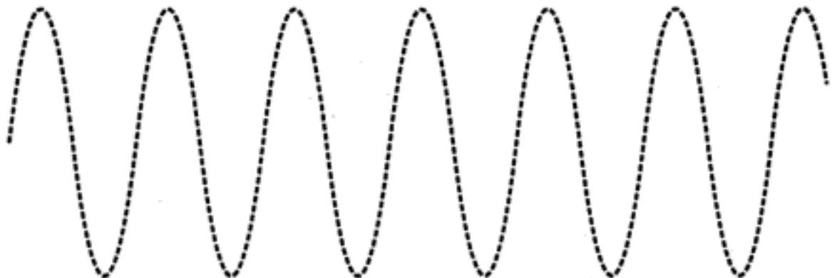
Fig. 2.12.2 A sine wave of frequency 10 Hz and sampled at 1000 Hz displayed on the screen
